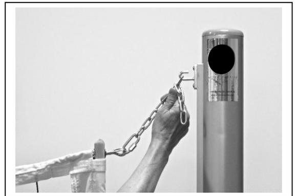
3. Turn the winch handle clockwise until adequate top cable tension is achieved. The winch should be about 2/3 of the way collapsed at this point. It is normal and desirable to have the posts bending inward slightly with the net under tension. This is known as deflection.
