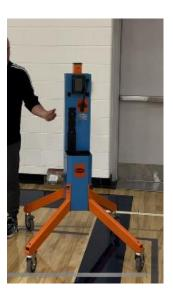
5) Place the ball launcher onto the main body. Attach and fully tighten the cords. Make sure the cord hangs straight down and that it is not caught between the main body and the ball launcher.
