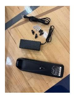
2) This is a cordless machine which uses an eBike battery. Begin by plugging the battery into the charger (just below on/off switch of battery), and fully charge the battery. Charging time may vary, but a full charge takes about 5 hours. NOTE: Some batteries come with a small round RCA jack for charging while some have a 3-pin XLR Cable for charging.
