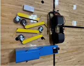
2) This is a cordless machine which uses a Sodium-Ion battery. Begin by plugging the base into the charger (flat shelf below the screen has a 3-pin XLR plug) and fully charge the battery. Charging time may vary, but a full charge takes about 5 hours. NOTE: Because this is a Sodium-Ion battery, there is not a risk to leaving the machine charging overnight – unlike a Lithium-Ion battery.
