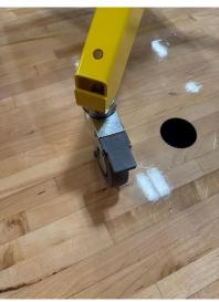
5) Locate the T-Handle and Bolt on the Ball Launcher. Push the Bolt through from inside of ball launcher and screw the T-Handle onto the bolt until tight. Place the ball launcher onto the main body. Attach and fully tighten the cords. Make sure the cord hangs straight down and that it is not caught between the main body and the ball launcher.
