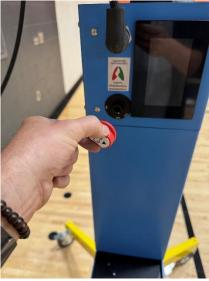
7) Turn the main power switch ON by rotating clockwise to 9 o'clock. Check the Ball Launcher to make sure there is nothing in or around the wheels, and then press the START button on the touchscreen.
